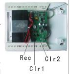
Delet coding: when need to delet the coding, press [Clr1][Clr2] key at the same time it will give a long sound "dee...", Then long sound again. Release [Clr1][Clr2] key, then you have delet all code address.
